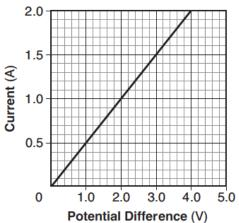
The resistance of the conductor is
