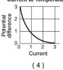
24. A long copper wire was connected to a voltage source. The voltage was varied and the current through the wire measured, while temperature was held constant. The collected data are represented by the graph below.
